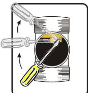
Cut PRONG to Release Water Pressure. Pry Tab with long #3 Phillips Screwdriver in a continuous motion
